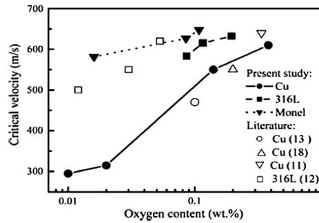
Fig. 5 Effects on Critical velocity with change in oxygen contents [7].
