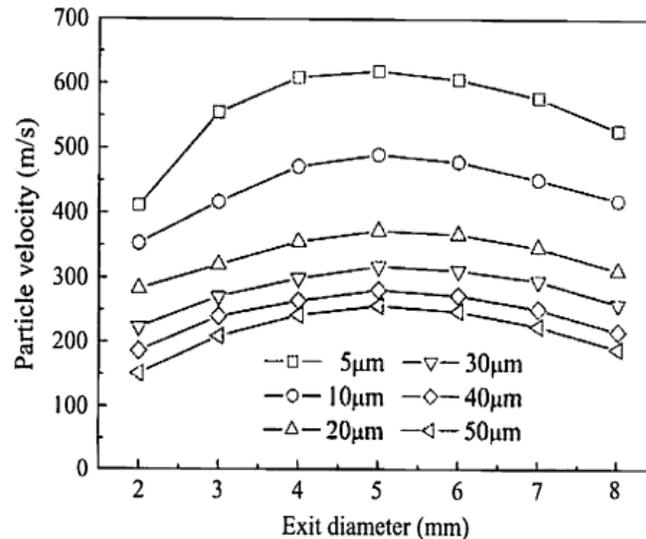
Fig. 6 Nozzle exit diameter Vs velocity of particles of different sizes [6].
