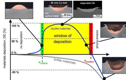
Fig. 1 Schematic diagram of the materials deposition efficiency (DE) as a function of impact velocity for a certain impact temperature [17].
