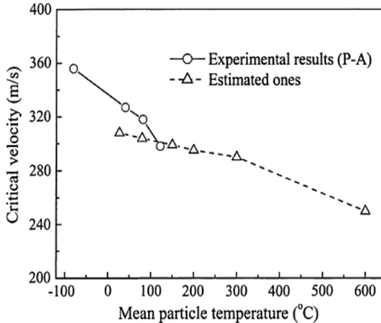
Fig. 4 Shows the variation of critical velocity with mean particle temperature [9].
