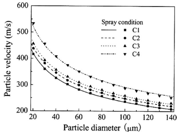
Fig. 3 Shows the variation of particle velocity with particle size under different spray condition [9].
